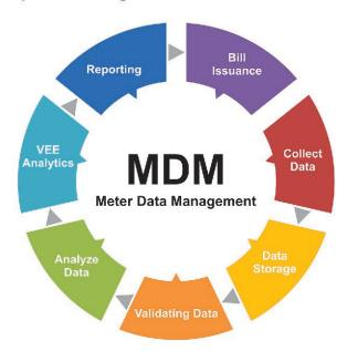
An MDM system will typically collect and import the data, then validate, cleanse and process it before making it available for billing and analysis. It also extends AMR technology by providing two-way meter communications, making it possible to send commands to the meter for various purposes including demand-response actions, time-based pricing (tariff) management and metering configurations.
